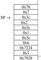
arraySum: lw a2, 0(a0) li a3, 1 beq a1, a3, end addi sp, sp, -8 sw ra, 0(sp) sw a2, 4(sp) addi a0, a0, 4 jal arraySum lw a2, 4(sp) add a2, a2, a0 lw ra, 0(sp) addi sp, sp, 8 end: mv a0, a2 ret
